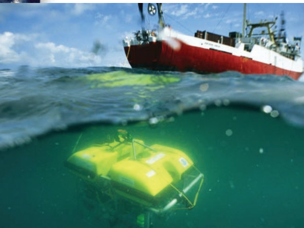
Tethered to the Star Hercules , the two-ton deep-sea camera sled Argo begins its descent three miles down below the surface to the dark cold where no sunlight penetrates. Right: Artist's rendition of Argo finding Bismarck .
